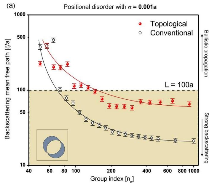
**Fig. 1:** Backscattering length calculated for different frequencies corresponding to different values of the group index in a valley and a conventional photonic crystal waveguide. The positions of the pillars have been randomized around their ideal values with a standard deviation of  $\sigma = 0.001a$ .
